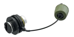
Benefiting from the expanded beam technology and the precision optical alignment the system creates high immunity against dust, mud, liquids and other contaminations. The FIBERFOX EBC25 2CH chassis connector converts a standardized LC patch cable into an expanded beam solution. It acts as a "feed-through" and has a jam-nut design.
